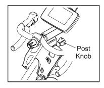
post, and firmly tighten the post knob. Make sure that the post knob is engaged in an adjustment hole. IMPORTANT: Do not adjust the handlebar post beyond the stop mark on the handlebar post.
