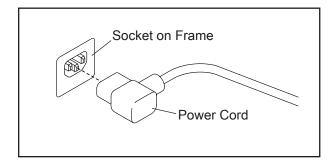
2. Plug the power cord into an appropriate outlet that is properly installed and earthed in accordance with all local codes and ordinances.
