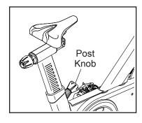
tighten the post knob. Make sure that the post knob is engaged in an adjustment hole. **IMPORTANT: Do not adjust the saddle post beyond the stop mark on the saddle post.**
